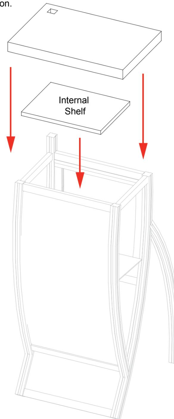
WHEN DISASSEMBLING TIGHTEN ALL KNOBS TO PREVENT LOSS DURING SHIPPING
